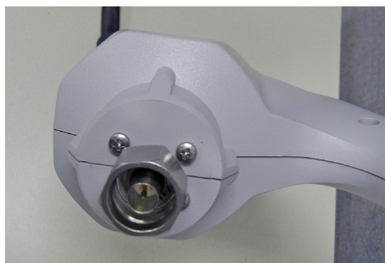
Figure 3-2. Remove the 2 Screws in the Top Half (Side with the Screw Holes) of the Case
